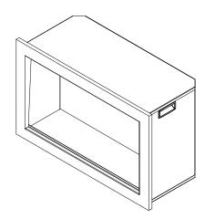
5. Put the fireplace into the wall opening and fix it to the wall by screwing 2 screws each side.
