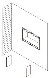
7. Insert the front glass panel back in place after the media installation has been completed.
